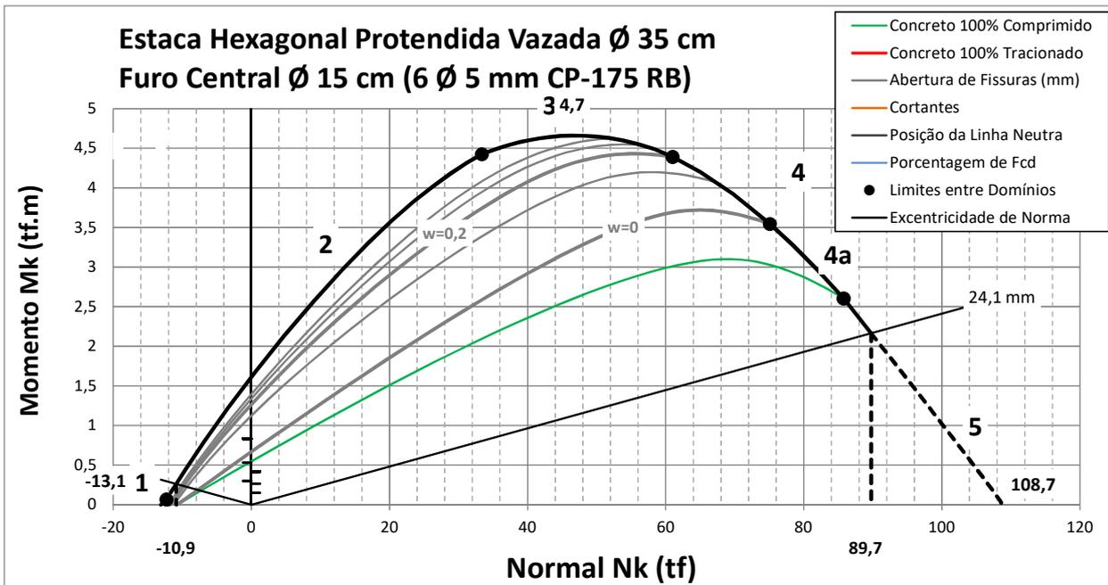
Nome: Estaca Hexagonal Protendida Vazada Ø 35 cm Furo Central Ø 15 cm (6 Ø 5 mm CP-175 RB)
